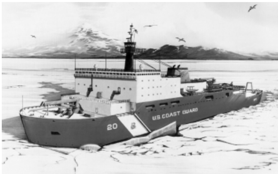
The USCGC Healy is a modern polar research vessel designed to be operated by the U.S. Coast Guard for the U.S. polar science community: 420' length, 28' draft, 30,000 HP, 4.5' ice at 3 knots; 4,000 sq. ft. of lab space including climate-controlled main lab and bio-chem lab, dry assembly area, wet lab, science refrigerator/freezers; electronics/computer lab, 4-season capability, science conning station, crew of 75 (14 in helo group), 4 sheltered lab/container vans; 35 science berths (surge capacity 50); 2 large out-of-weather 'garage' staging areas, diving support, uncontaminated seawater system, fiber-optic computer/video/data net, and multi-beam sonar (illustration courtesy of Guy Tapper).
