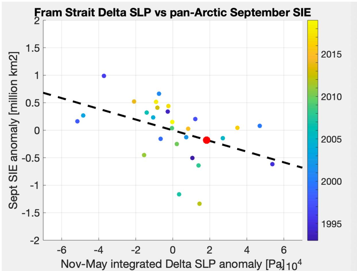
Scatter plot of the anomaly of the time integrated sea level pressure difference between Greenland and Svalbard and the anomaly of the mean pan-Arctic September sea ice extent. The coefficient of correlation between the two is  $r=-0.45$ . The dashed line represents the best linear fit going through zero. The red dot indicates the sea level pressure difference anomaly for 2020.
