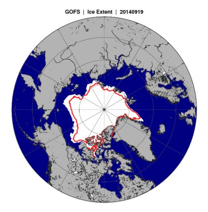
**Figure 4:** Spatial forecast map of the projected GOFS 3.1 September minimum ice extent for 19 Sept 2014. White area indicates ice concentrations > 15% in the uncorrected simulation. The red line represents the bias-corrected predicted ice extent of 4.5 Mkm<sup>2</sup>. This represents the 55% concentration isoline.
