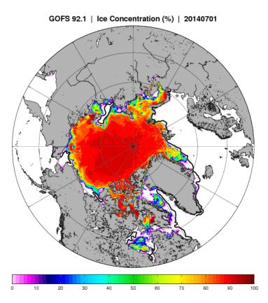
**Figure 1:** Ice concentration field (%) from GOFS 3.1 valid July 1, 2014. This is the initial condition for each ensemble member. The black line on the figure represents the independent ice edge provided in real time by the National Ice Center.
