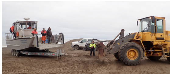
Heavy equipment being used to launch a boat big enough for large waves but too big for the boat ramp when the water is low at Utqiagvik, Alaska
