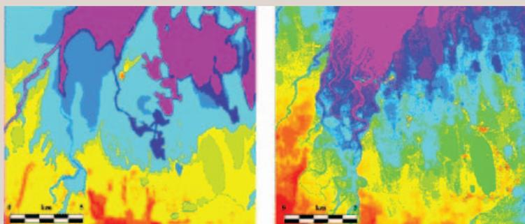
*A portion of the Kuparuk River watershed shown with the standard USGS DEM data (left) compared with the new, high resolution data (right). Figures courtesy of Matt Nolan.*
