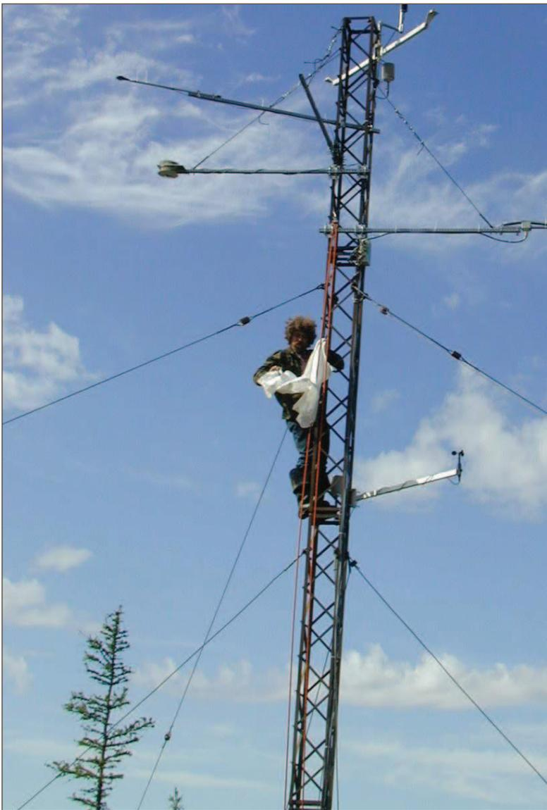
*Sergei Zimov finishes installing instruments on an eddy flux tower near the Northeast Science Station in Cherskii, Siberia. Photo courtesy of VECO Polar Resources.*
