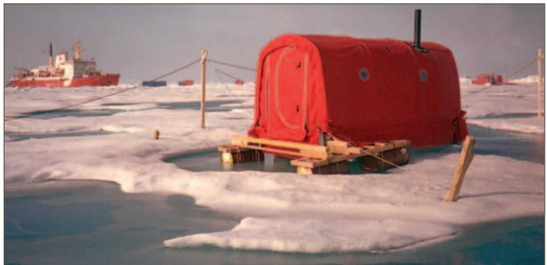
*During the summer of 1998, SHEBA investigators had to float instruments and structures on barrels when the ice melted out from under them. Photo courtesy of University of Washington.*
