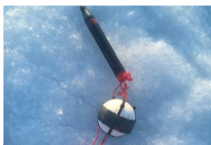
Fig 1 – Cryoegg ready for deployment at Store Glacier
