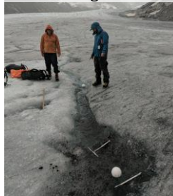
Fig 4 – two Cryoeggs used for salt tracing in a stream
