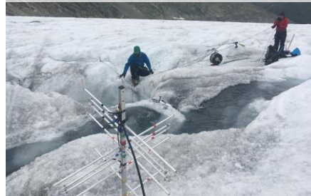
Fig 5 – Cryoegg deployment in an artificial moulin on Rhône Glacier
