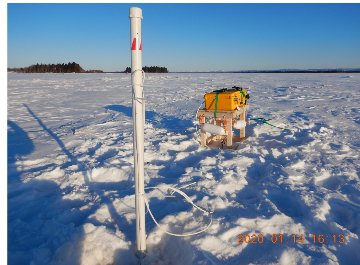
Figure 2. The photograph is of an ice monitoring unit installed at site number 3 (see Figure 1). The yellow case contains the hardware (Battery, CPU, GPS, Iridium transmission etc.). It is mounted on a raised pallet to reduce the risk of it being buried by a heavy snowfall. A string of thermistors is connected to the yellow case and attached to the vertical white pipe (in the foreground) that is installed into the ice through a borehole. The thermistor string subsequently freezes in situ such that a temperature profile of the air/snow/ice/water environment can be derived (see Figure 3). The system is usually recovered at the end of the season once the thermistor string melts out but whilst the ice is still safe. If the unit cannot be recovered it has flotation such that it can be recovered from boat, if it survives the break-up.
