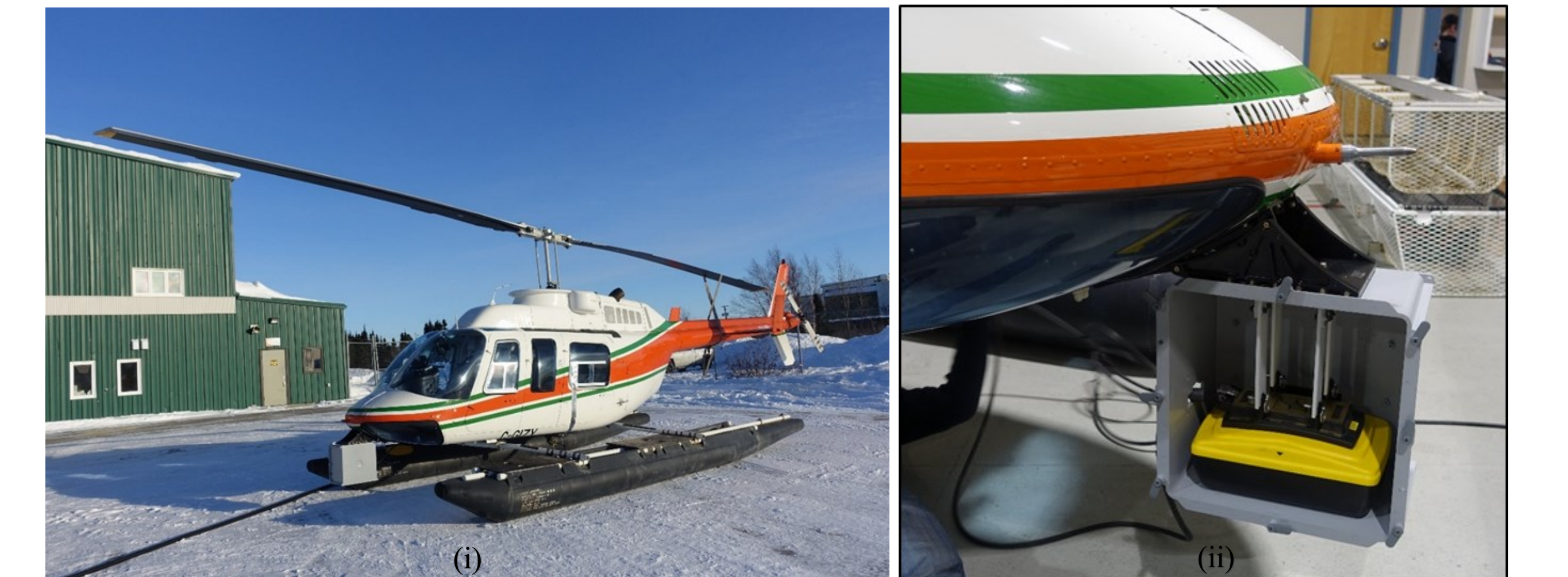
Figure 7. (i) Universal Helicopters Bell 206L, with floats, on the apron at Universal Helicopters' Goose Bay hanger. The grey box on the front is the GPR mount enclosure. (ii) GPR transmitter/receiver (yellow box) mounted inside the enclosure (grey case) attached, using a G1 camera mount, to the nose cowling of the helicopter (a side panel is attached to seal the enclosure prior to flight).
