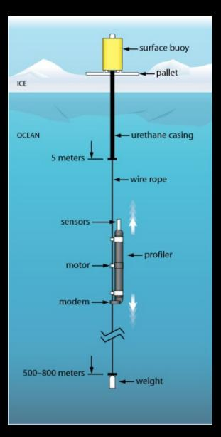
ITP: autonomous profiler system to measure water column property profiles under perennial sea ice.Like Argo float, except tethered to a cable in ice.Typically 4x profiles per day over the top 800m.
