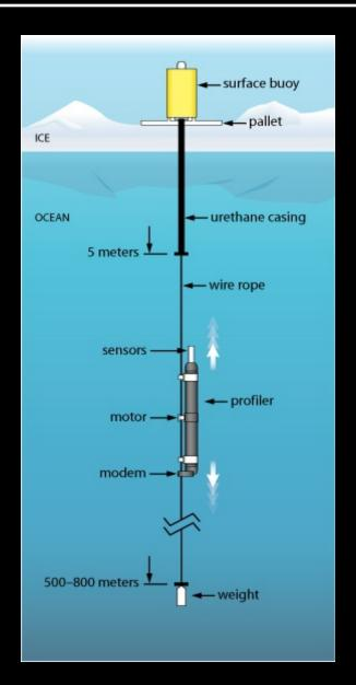
ITP: autonomous profiler system to measure water column property profiles under perennial sea ice.
