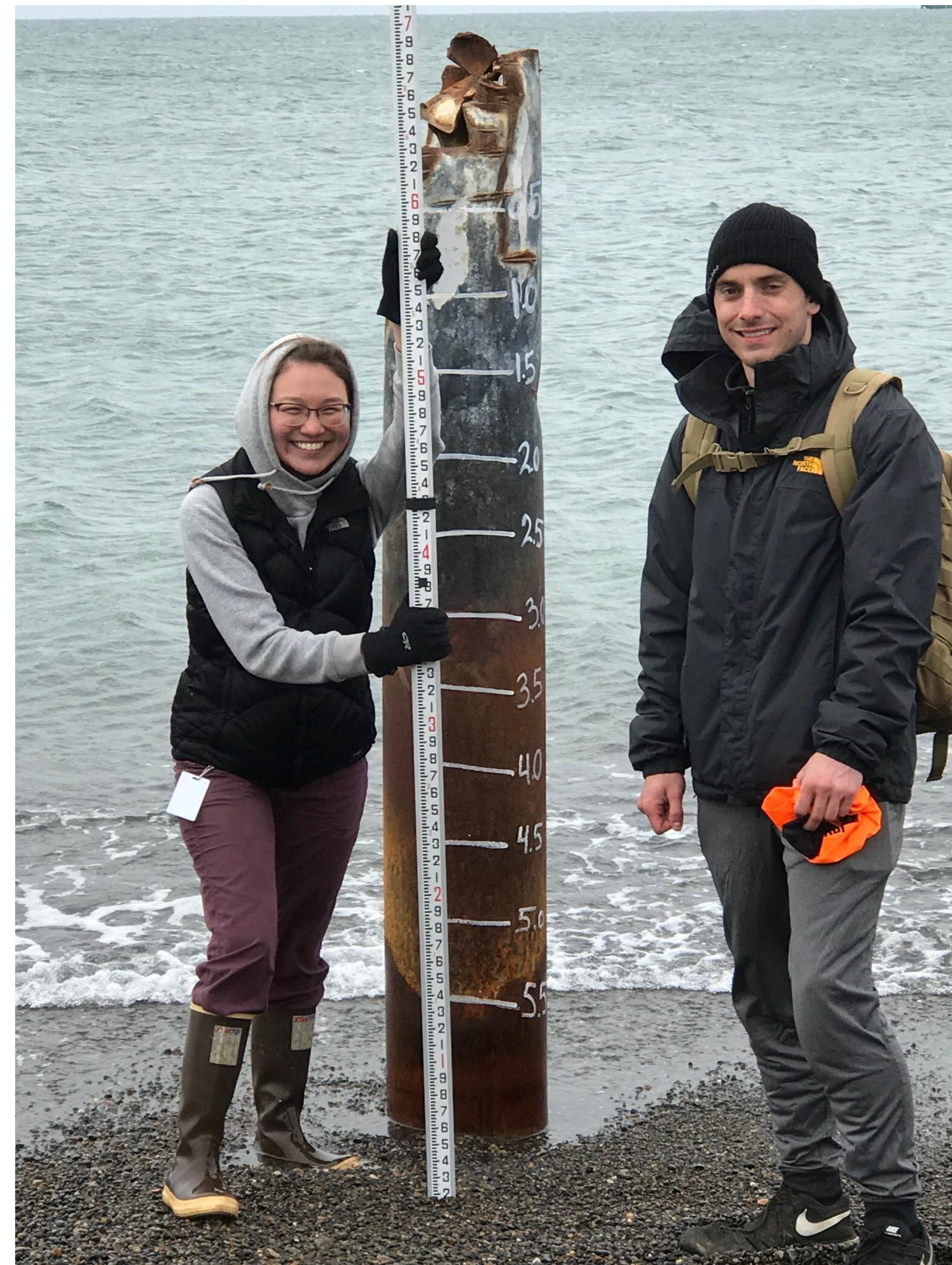
Beach surveying and water level/wave monitoring at Utqiagvik (Barrow) Alaska
