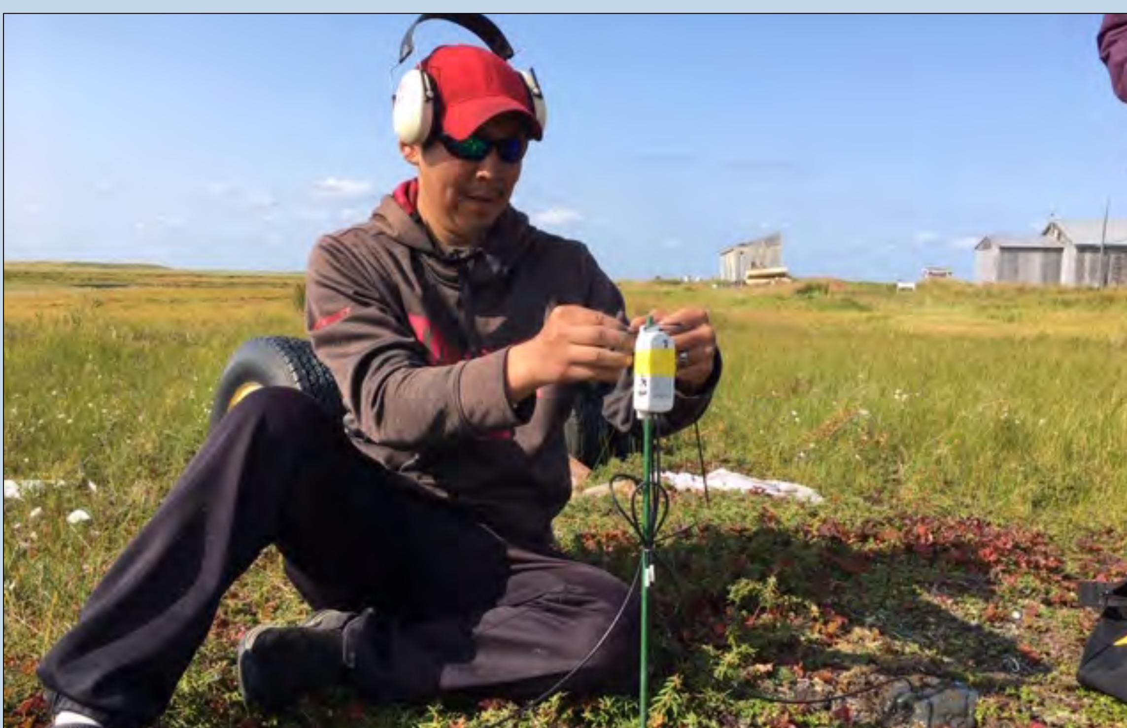
Lewis Amik installing temperature sensors for permafrost monitoring.
