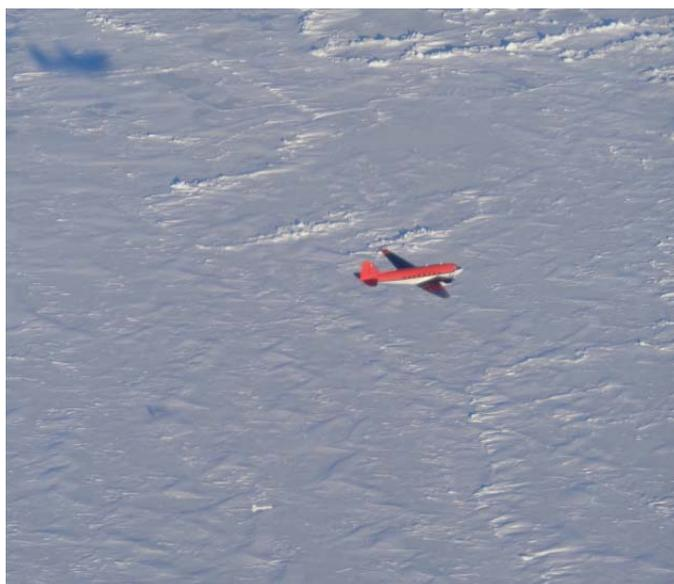
**Figure 1:** York University's Airborne Sea Ice Observatory (ASIO) with tethered AEM ice thickness sensor (white torpedo near left/central lower margin). Note shadows of aircraft and sensor. Photo courtesy Mark Drinkwater, ESA@CryoVEx 2014.
