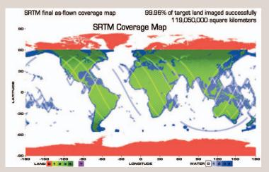
The figure shows the coverage of radar elevation measurements taken from the space shuttle Endeavour in 2000 during the Shuttle Radar Topography Mission. These measurements provide publicly available high resolution Digital Terrain Elevation Data for most of the globe. Note the absence of data in the Arctic. Similar data are available for the Antarctic region from the 1997 Radarsat Antarctic Mapping Project. Map from www.nima.mil/cda/article/ 0,2311,3104\_10579\_112959,00.html.
