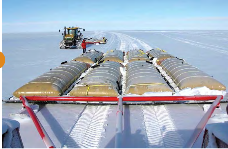
Figure 11. Tractor and fuel bladders on the overland traverse. Source: Paul Thur.
