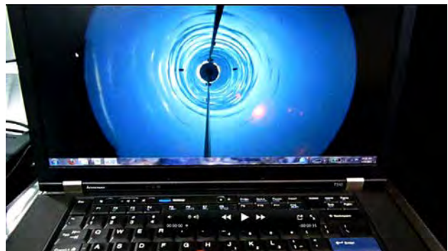
An image from the Whillans Ice Stream Subglacial Access Research Drilling project (WISSARD) borehole camera. In January 2013, scientists and drillers with this interdisciplinary project announced that they had successfully used a first-of-its-kind, biologically-clean hot-water drill to directly obtain samples from the waters and sediments of subglacial Lake Whillans. Credit: The Whillans Ice Stream Subglacial Access Research Drilling Project
