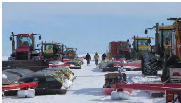
Long-distance, over-snow, heavy-haul traverse trains provide an efficient alternative to airlift for moving cargo, fuel, and science equipment to remote sites. Credit: The Whillans Ice Stream Subglacial Access Research Drilling Project
