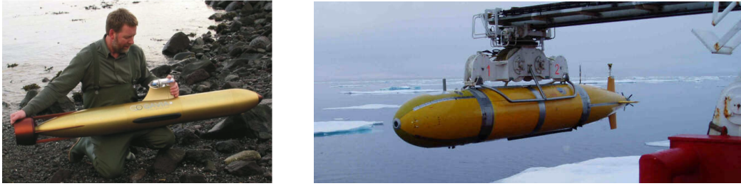
Fig. 4: (a) Gavia person portable AUV and (b) Autosub long-range AUV hanging from its shipboard overboarding system.
