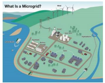
Schematic of a community microgrid (ACEP 2015). Microgrids include energy sources, the power lines that distribute electricity, and energy sinks.
