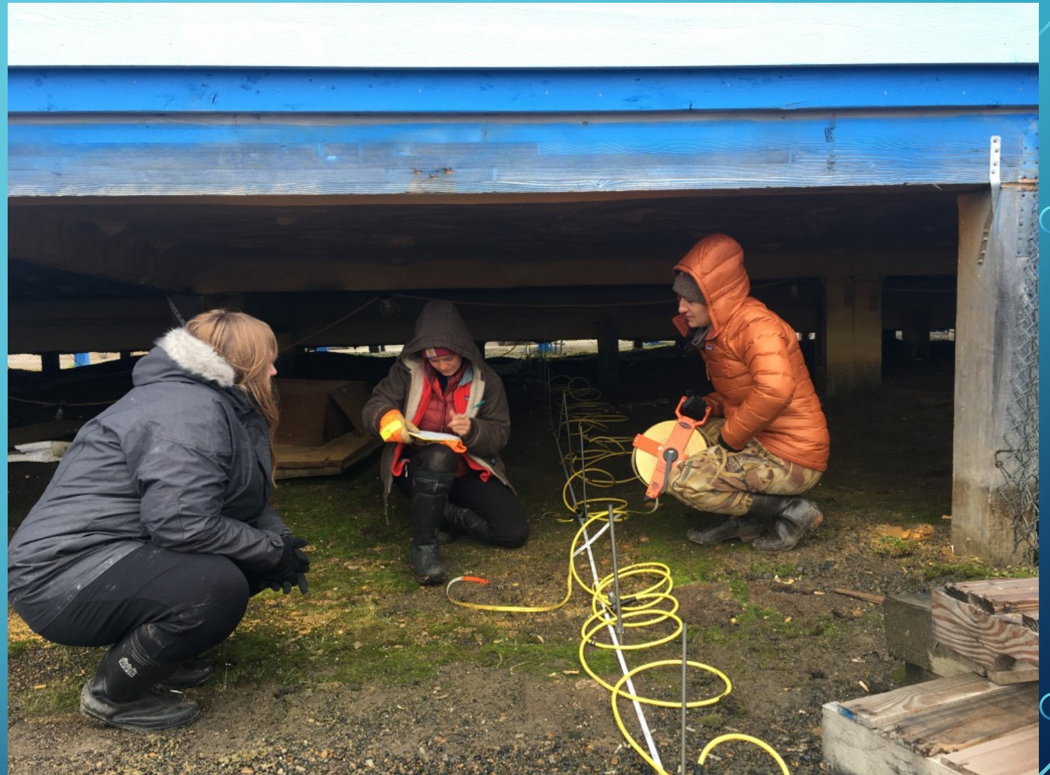
Ground Penetrating Radar and Electrical Resistivity Tomography to measure active layer and ground ice (UVA and CRREL)
