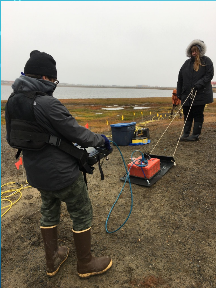
Ground Penetrating Radar and Electrical Resistivity Tomography to measure active layer and ground ice (UVA and CRREL)
