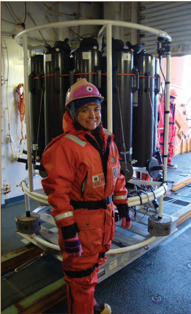
Chantelle Rose with the CTD (Conductivity, Temperature, and Depth instrument). Aboard the USCG Cutter Healy. Photo by Joel Llopiz, courtesy of Chantelle Rose, courtesy of ARCUS.
