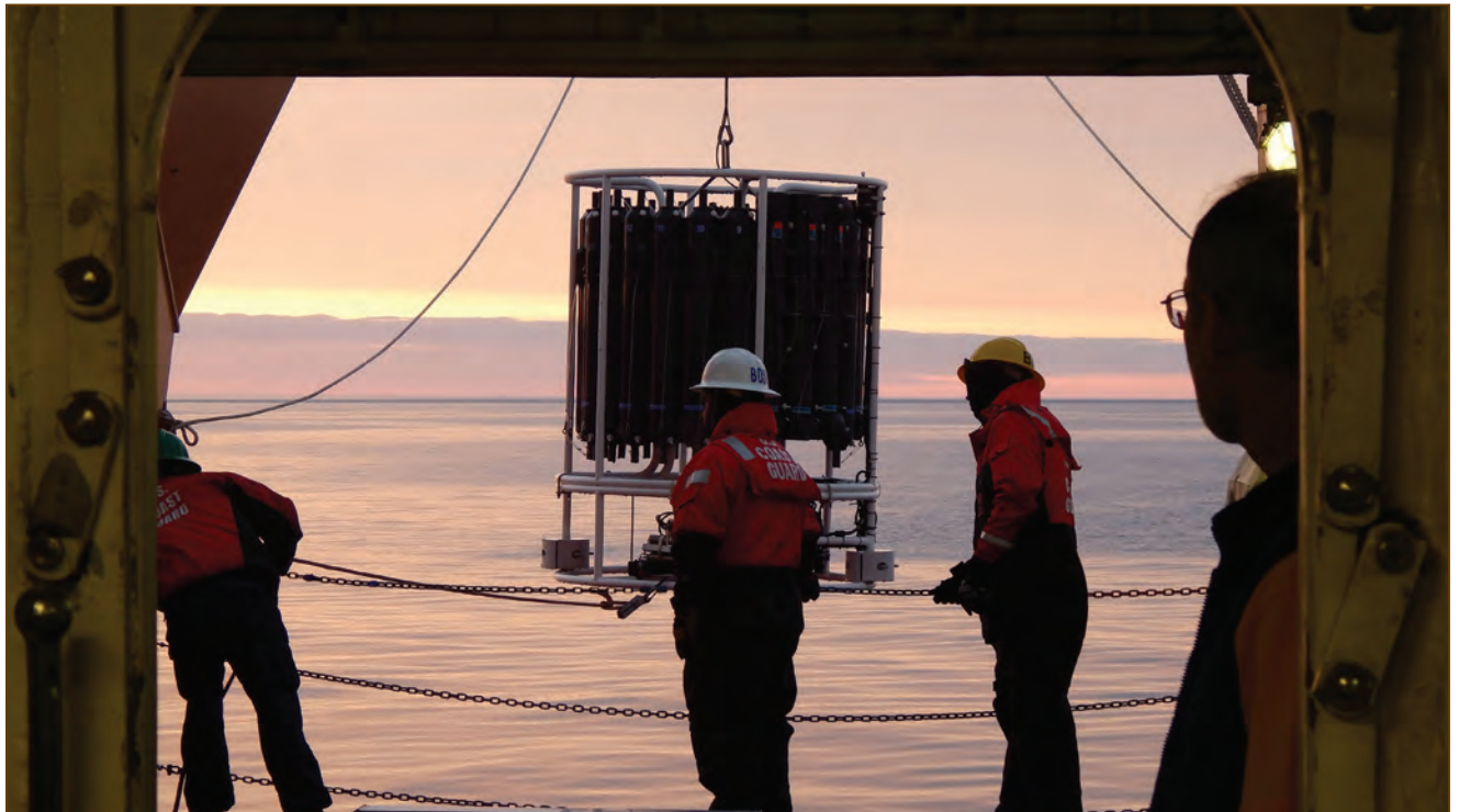
The CTD (conductivity, temperature, and depth instrument) at dusk. Aboard the USCGC Healy on the Chukchi Sea. Photo by Andrea Skloss, courtesy of ARCUS.
