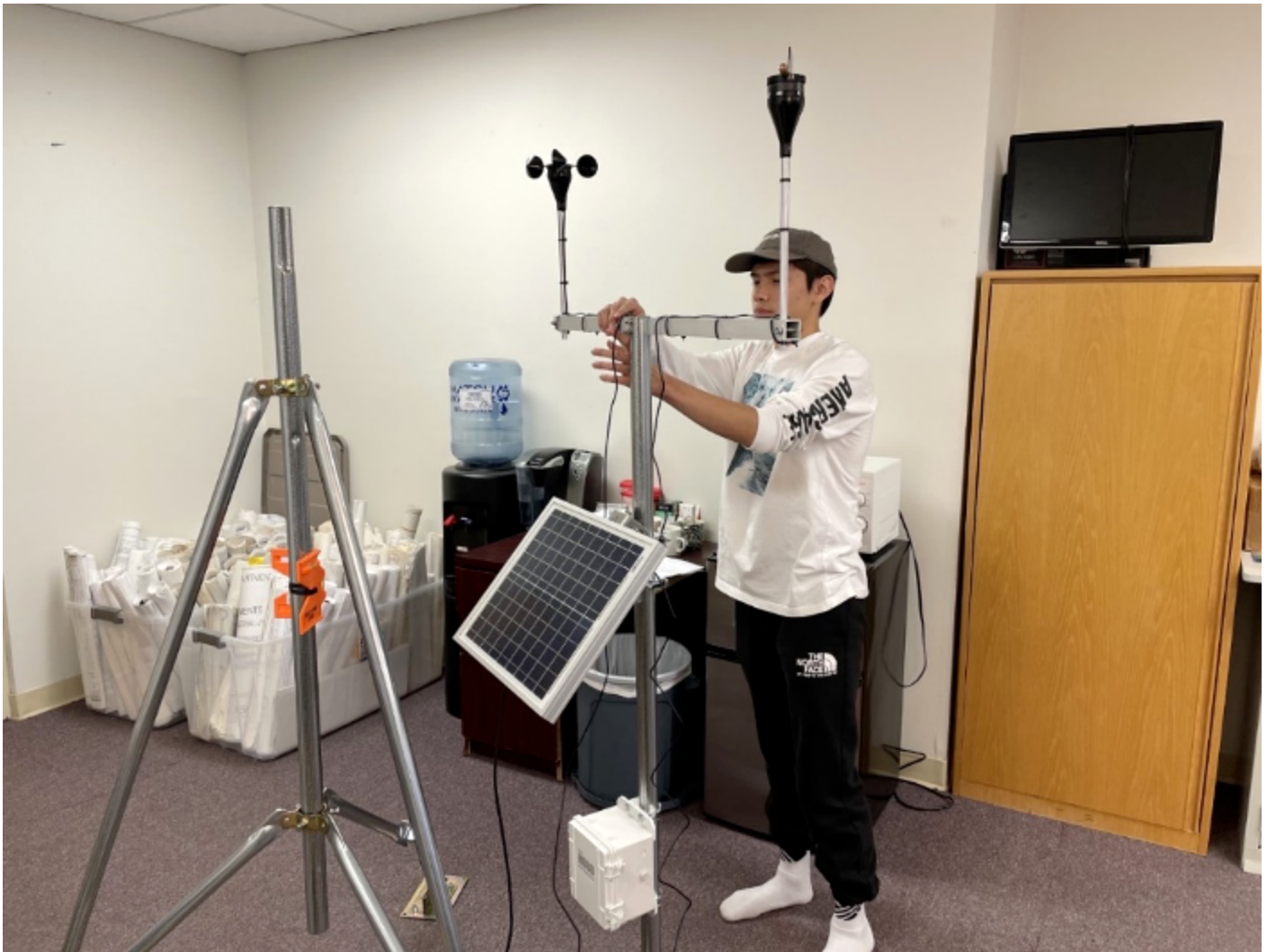
Figure 4. Mikal Nelson erecting an environmental sensor station at the TRIBN office in Utqiagvik. Photo courtesy of Lars Nelson.
