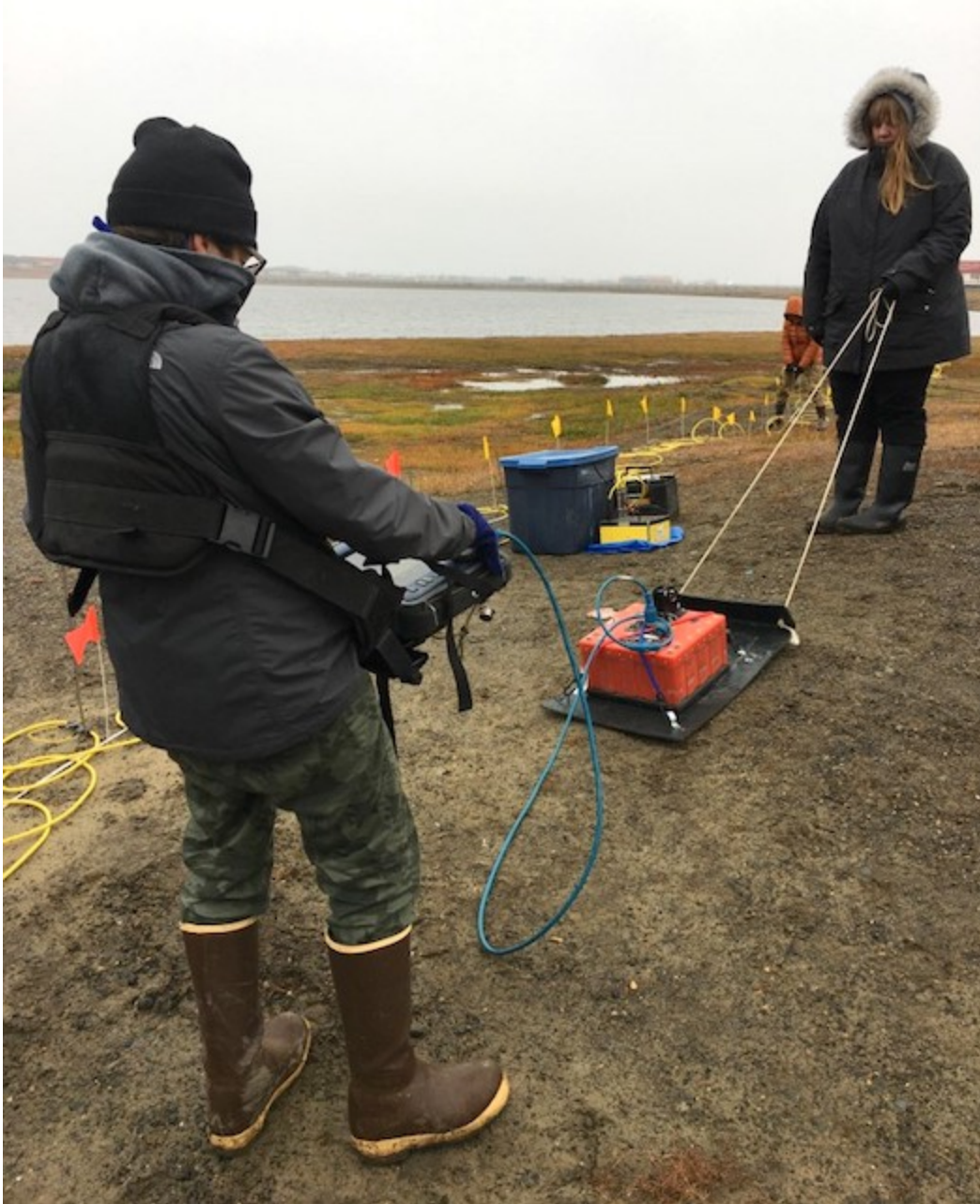
Figure 2. Team members conducting ground penetrating radar (GPR) at different locations within Utqiagvik, Alaska. Photo courtesy of Luis Felipe Rosado Murillo.
