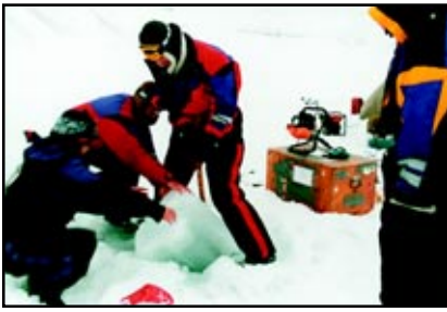
Extracting an ice core from a hydro-hole for turbulence studies under fast ice in Temple Fjord, Svalbard, March 1999. Photo by S. McPhee.
