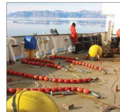
UD researchers prepare to deploy one of eight conductivity-temperature-depth strings from the deck of the CCGS Henry Larsen in Kennedy Channel between Greenland and Ellesmere Island, Canada, as part of an NSF-supported project investigating arctic freshwater flux. The instruments provide time series of temperature and salinity as a function of depth. The red capsules float above the larger yellow buoys (moored at a depth of approximately 200 meters) and allow the mooring to slide smoothly through the crevices of icebergs that can have drafts of up to 150 meters. Photo courtesy of Andreas Muenchow.
