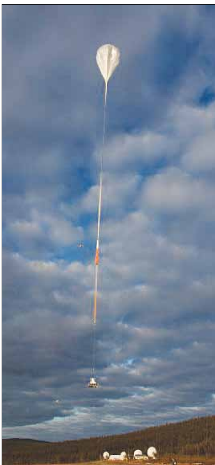
Launch of the Anti-Electron Sub Orbital Payload instrument from NASA's Columbia Scientific Balloon Facility in Kiruna, Sweden, in June of 2006. This balloon is made of a polyethylene film (the same type of material used to make trash bags), weighs approximately 5,000 pounds, and can carry an 8,000-pound load. Photo by Andrew McDermott.
