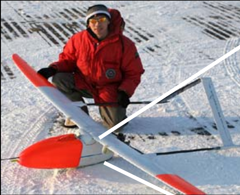
Riming on wings of an Aerosonde robotic aerial vehicle
